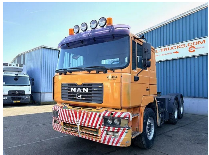
MAN 26.463 DFS 6x4 FULL SPRING SUSPENSION TRACT...
